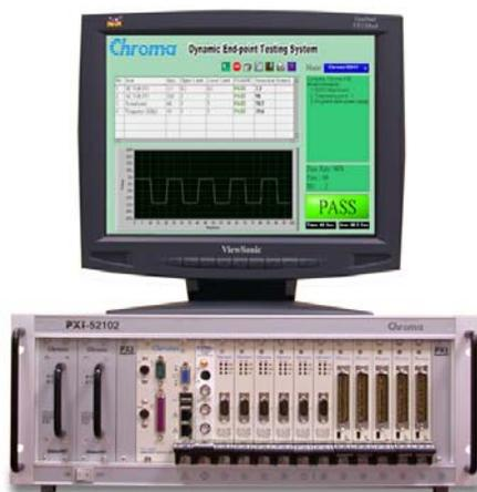
Figure 8. PCB Automatic Test System
