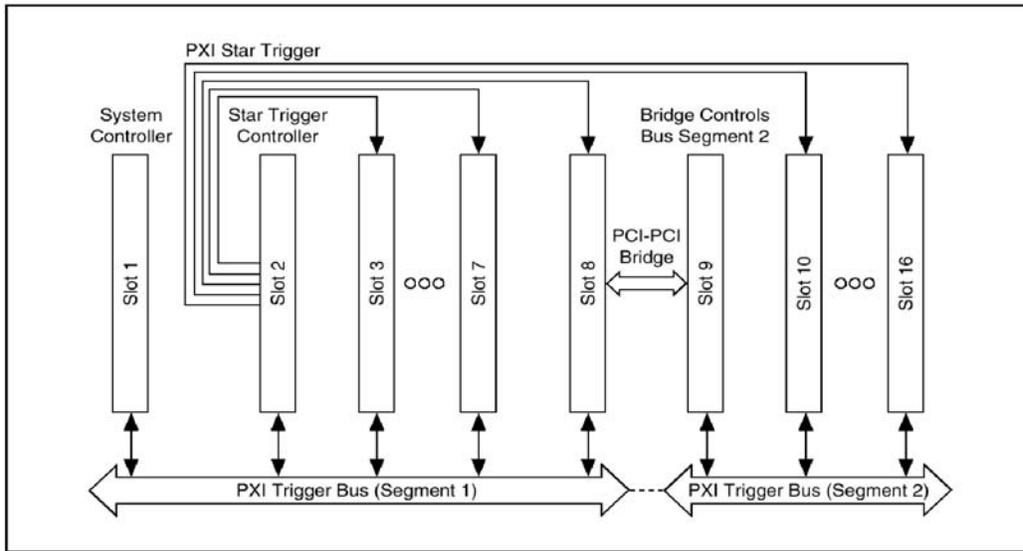
**Figure 5.** This block diagram from the PXI standard shows the implementation of the PXI Trigger Bus and of the PXI Star Trigger. The trigger bus has eight bidirectional lines to each slot. The Star trigger has a dedicated line between slot two and each of the other slots in a chassis. Special slot two modules have the ability to bridge the trigger lines to an additional chassis
