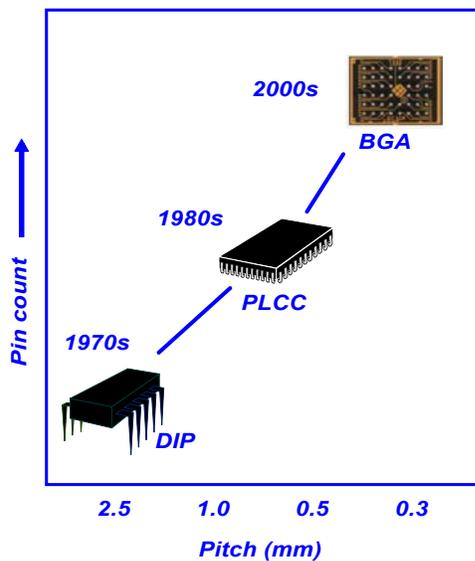
**Figure 6.** Trend in IC device complexity
