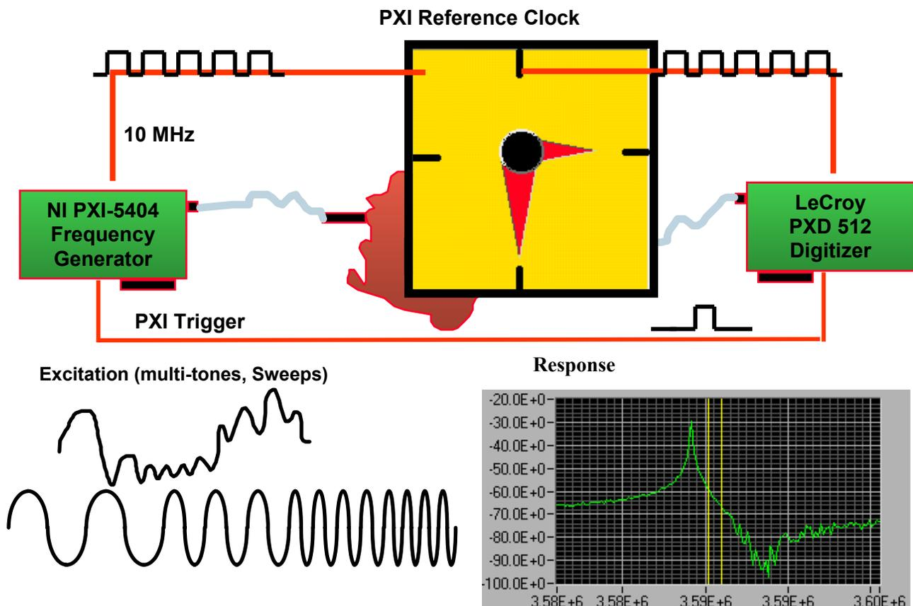
Figure 2. PXI as a Signal Source Platform
