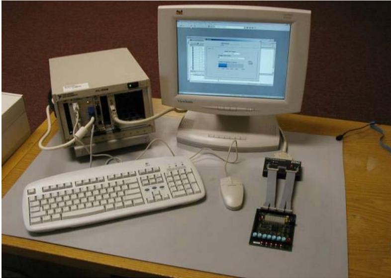
**Figure 7.** Functional test system, including PXI-based boundary-scan controller for structural Testing
