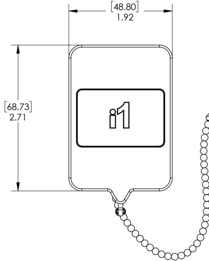
ATTACH FREE END OF THE LANYARD TO DESIGNATED LOCATION ON RECEIVER. LANYARD CAN BE PERMANENTLY REMOVED AND DISCARDED IF DESIRED.
