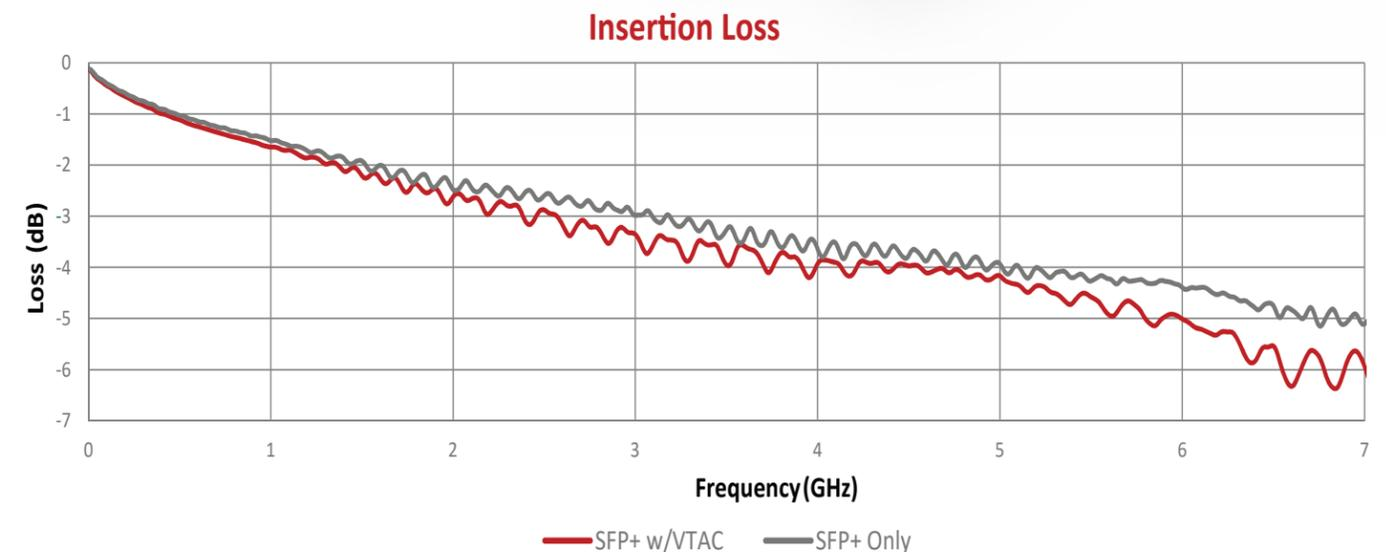
Insertion loss was tested on one-meter long patchcords with SFP+ terminations on either end. The second data line shows the same patchcord that has been bisected and terminated with VTAC connectors in its center.
