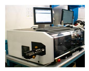
VPC's state-of-the-art wire cut and strip machine provides accurate and precise tolerances with each cut and strip.
