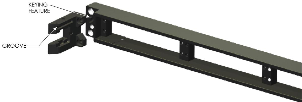
The rotation blocks were also designed with a tongue and groove feature to prevent placing the ITA in upside down.
