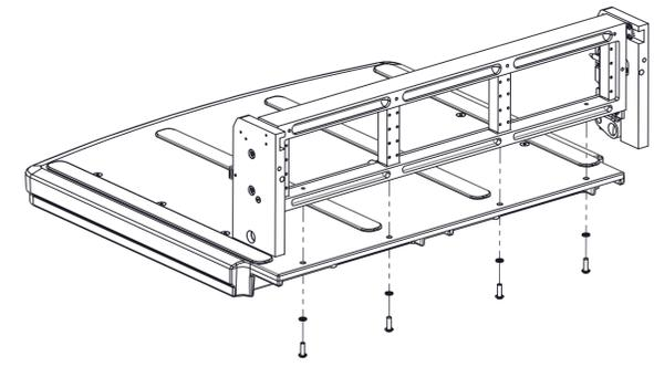
310104408-1 PLATFORM ASSEMBLY. HANDLE AND TORSION SHAFT NOT SHOWN FOR CLARITY
