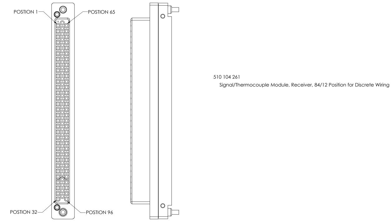
Thermocouple Contacts occupy the bottom 12 Positions
