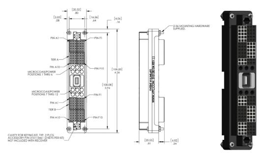
Hybrid version of i2 Micro iCon offers 144 QuadraPaddle<sup>tm</sup> signal pins and 6 micro coax pins
