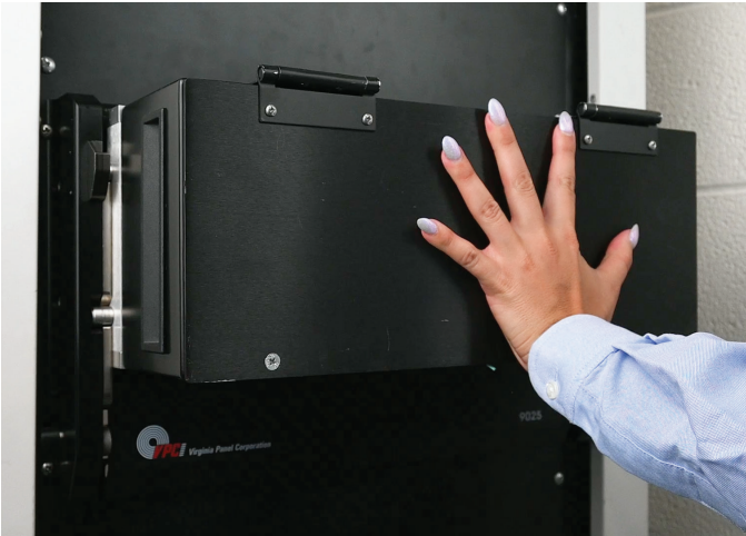
Figure 5: Applying pressure to the top of the ITA
