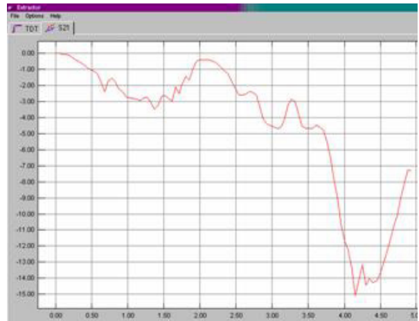
Figure 2. 16" Blue cable female Z-Trace to male VP to female Z-Trace with cable and Z-Trace connectors de-embedded (-3 dB at 1.2 GHz)
