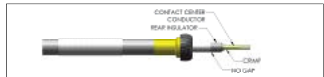
Figure E. Make sure there is no gap between the center conductor and the dielectric.
