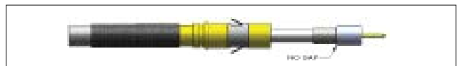
Figure F. Make sure there is no gap between the front and rear insulators.
