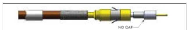
Figure G. Make sure there is no gap between the front and rear insulator.
