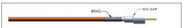
Figure F. Make sure there is no gap between the rear and front insulator.
