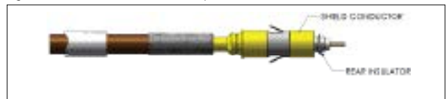
Figure E. Install shield conductor and rear insulator.
