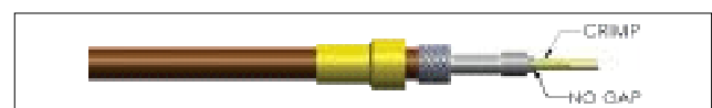
Figure F. Make sure there is no gap between the center conductor and the dielectric.
