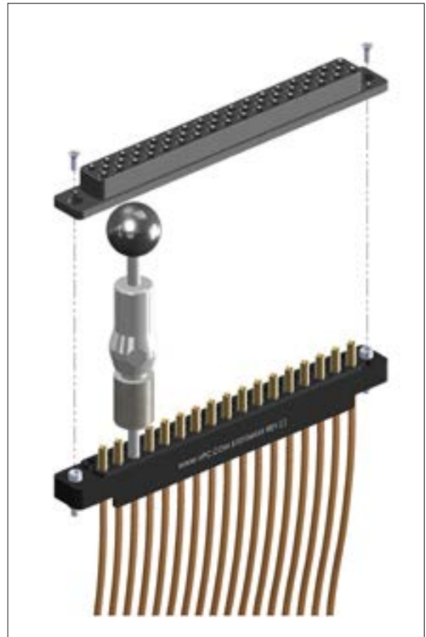
Figure A. Ensure that the tool is kept perpendicular to the module face to avoid damage to the contact or tool.
