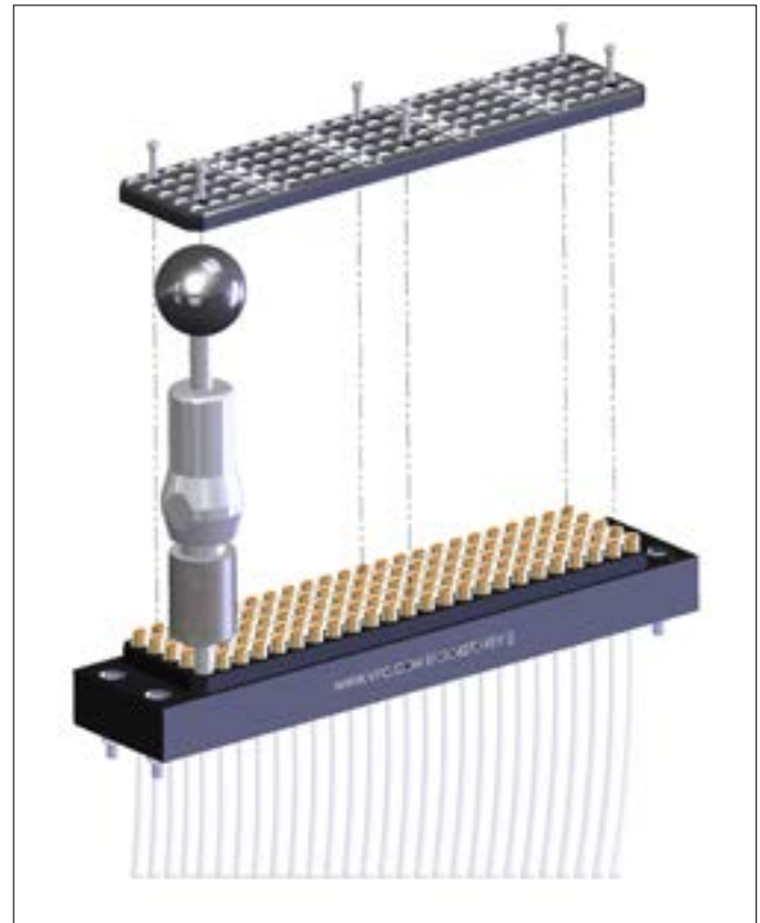
Figure A. The Micro Power module has six 0-80 screws to be removed. Ensure that the tool is kept perpendicular to the module face to avoid damage to the contact or tool.
