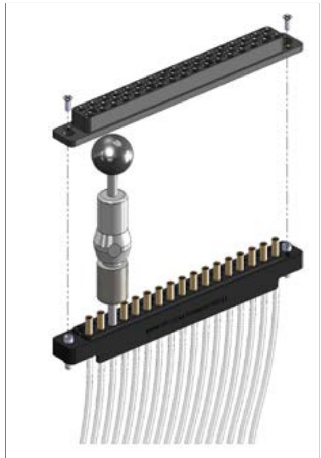
Figure A. Ensure that the tool is kept perpendicular to the module face to avoid damage to the contact or tool.
