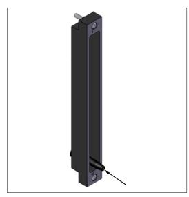
Figure C. Press contact out of module.
