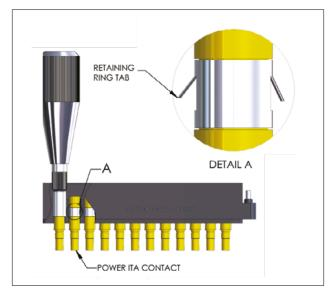
Figure B. Fully seat the tool before pressing down.
