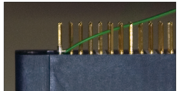
Figure B. Completed wrapped wire.
