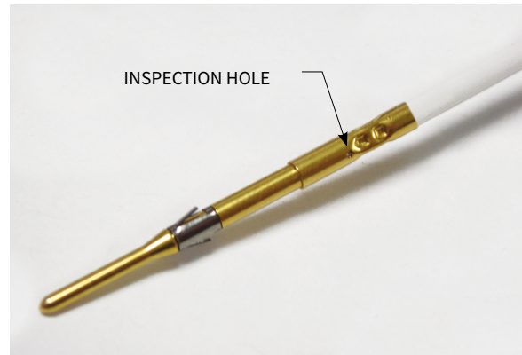
FIGURE B. The crimp region is between the inspection hole and the end of the contact (610110129).
