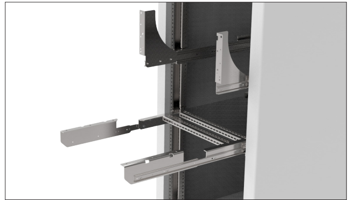
Figure F. Attach platform mounting flanges to the inner slide rails.
