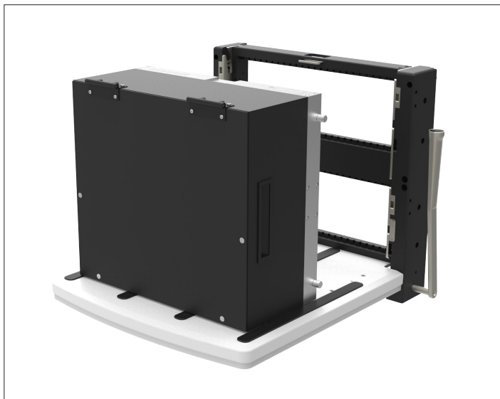
Figure A. Enclosures must be flush with the bottom of the ITA frame to ensure mating with the 9050TR receiver. The width of the enclosure may grow with customer needs, as long as the extended width is offset to the side opposite the engagement handle. There is no limit to the height of the enclosure.
