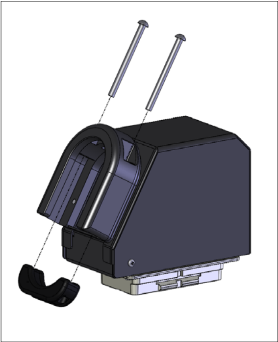
Figure E. Slowly alternate tightening the screws until the clamp has closed the wires or cables securely.
