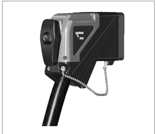
Figure B. The eyelet coupling can be used to attach the protective cover to the ITA using the 6-32 screw on the cable clamp.
