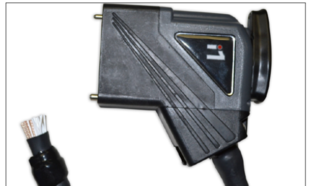
Figure B. Example of silicone tape usage.
