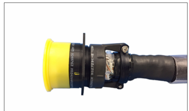
Figure C. Example of silicone tape on circular connector.
